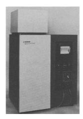
Ionics, Inc., Instrument Division is producing its LAB/1200 series of automatic analyzers for laboratory measurement of TOC, TOD, and TC. The analyzers, with prices starting at \$5,900, include digital electronic sequence for automatic unattended operation, automatic zero function to eliminate base line drift, all-ceramic sample injection valve, and rapid reponse times. Information: Ionics, Inc., Instrument Division, 65 Grove St., Watertown, MA 02172.
