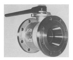
Marwin International Operations Ltd. is marketing a precision ball valve that includes a special fire-safe design: if the gland seal material burns out, the ball will seal against a special lip inside the ball casing to prevent leaks. Information: Marwin International Operations Ltd., Barkby Road, Leicester LE4 7LL England (tele: 0533-760181).
