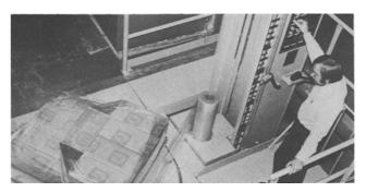
Reynolds Metal Company has introduced Reynolon SPOW (Stretch Pallet Overwrap), a 75 gauge polyvinyl chloride film, for application to loaded pallets while under tension. Information: Reynolds Metal Company, P.O. Box 239, Brookfield, IL 60513.
